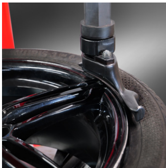
SHOWN: Lifting roller demounting lower bead
