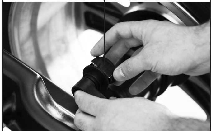
Fig. 31 Fit the adhesive weight in the pliers of the gauge rod
