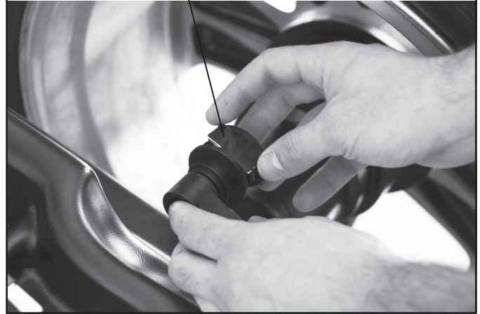
Fig. 37 Fit the adhesive weight in the pliers of the gauge rod
