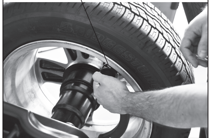
Fit weight on the position where weight pliers touches the wheel Fig. 38
