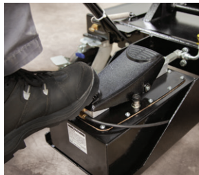
Push rear of foot pedal to raise table
