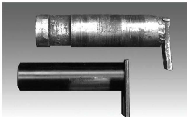
TOP PIN With Excessive Scoring and Wear
