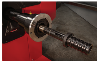
AIR BRAKE An electro-pneumatic brake keeps the wheel in the unbalance position.
