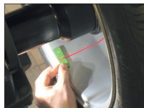
LASER BLADE The laser pointer indicates the exact positioning for weights
