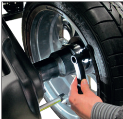
Automatic storage of distance and diameter.
