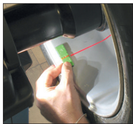
INTERNAL DATA ARM AUTOMATICALLY MEASURES RIM RUN-OUT
