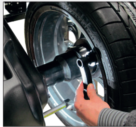
INTERNAL DATA ARM AUTOMATICALLY MEASURES RIM RUN-OUT
