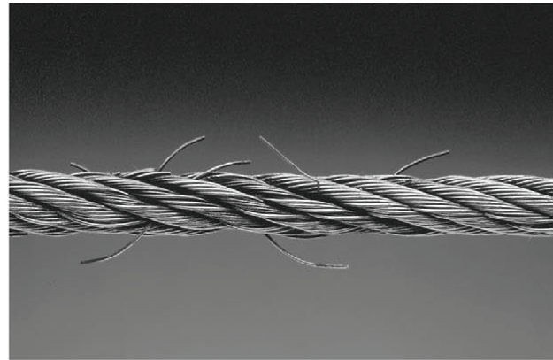
Cable With Broken Wires
