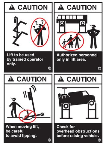
The messages and pictographs shown are generic in nature and are meant to generally represent hazards common to all automotive lifts regardless of specific style.
