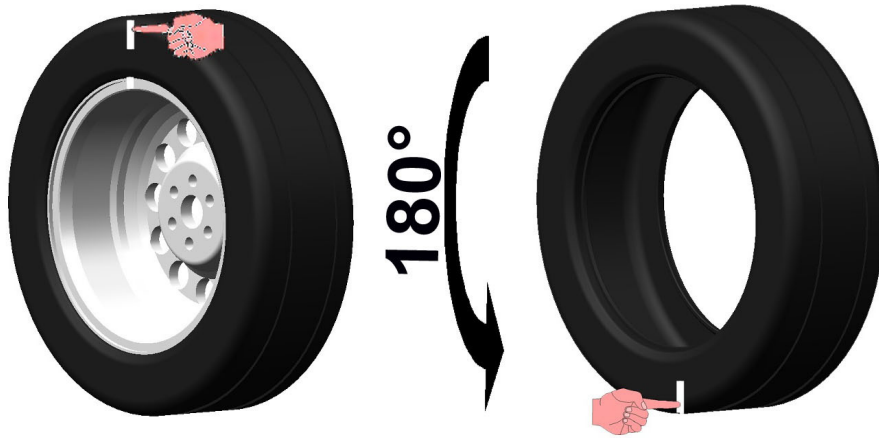
Fig. 72 Position the reference mark on the rim in line with the arrow on the flange
