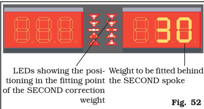
Upon reaching the correct position, the wheel is locked independently.
