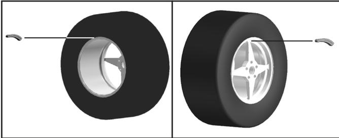
Once the wheel has been correctly positioned, fit the weight indicated by the machine on both sides of the wheel. The program automatically indicates the best weights to be fitted and rounds these off according to their position.
