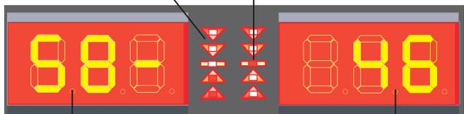
% value of the possible unbalance reduction compared to wheel current situation
