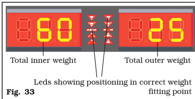
Once the unbalance value of the inner and outer wheel side is known, the wheel can be positioned by turning it in the direction indicated by the LEDs until the correct position is reached (see Par. 15.3.6).
