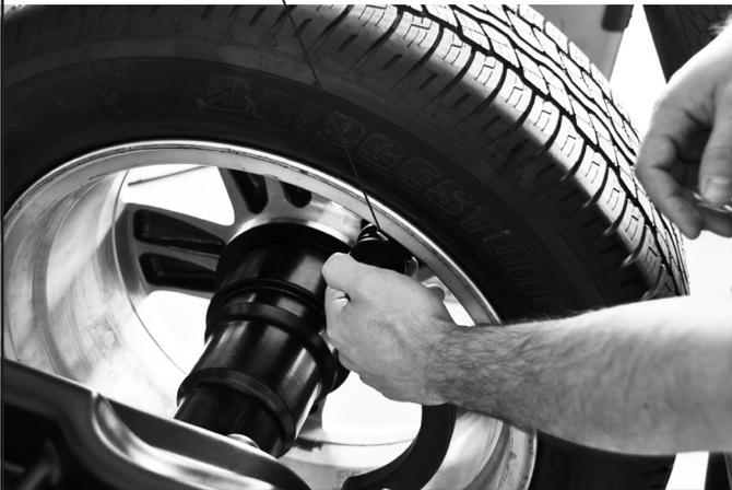
At the end of the procedure, the wheel balancing conditions can be checked by performing a trial spin. If the adhesive weight has to be hidden behind spokes, refer to "weights hidden behind spokes mode", (see Chap. 18).
