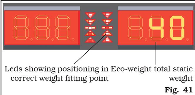
The wheel can be positioned by turning it in the direction indicated by the LEDs until the correct position is reached (see Par. 15.3.6).
