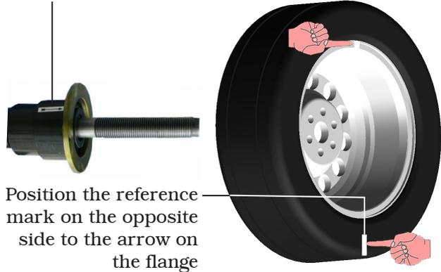
Position the reference mark on the opposite side to the arrow on the flange
