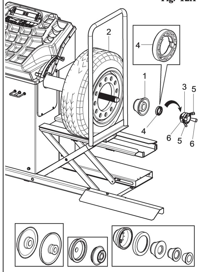
In case of wheels with peculiar sizes and features, the wheel has to be fitted onto the mandrel according to the previous instructions, however, the accessories (**Fig. 12B ref. 1-2-3-4**) shown in **Fig. 12B** shall be used.
