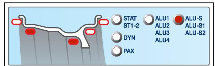
The ST2 function is a procedure that offsets wheel vibrations using a single adhesive weight on a single plane positioned exactly at 12 o' clock.
