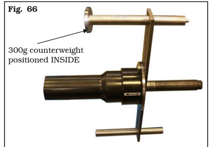
Press key to make a wheel spin with 300 g on the inner side.
