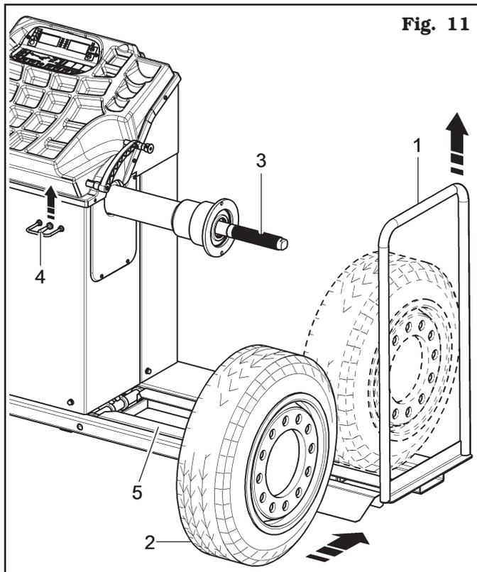
3. Place the wheel (**Fig. 11 ref. 2**) on the wheel support (**Fig. 11 ref. 1**) with rim inner side towards the wheel balancer. Operate the lifting device control (**Fig. 11 ref. 4**) and, keeping it lifted, lift the footboard (**Fig. 11 ref. 5**) and centre manually the wheel on the mandrel, with a minimum strain independently from its weight.
