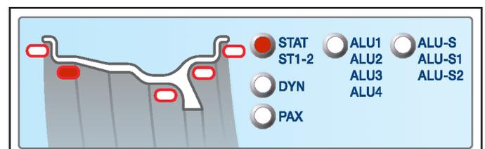
The ST1 function is a procedure that offsets wheel vibrations using a single weight with clip on a single plane positioned exactly at “12 o’ clock”. Enter the measurements (see Par. 15.1) and proceed as described in Par. 15.3.3 Dynamic balancing (only for wheel inner side).
