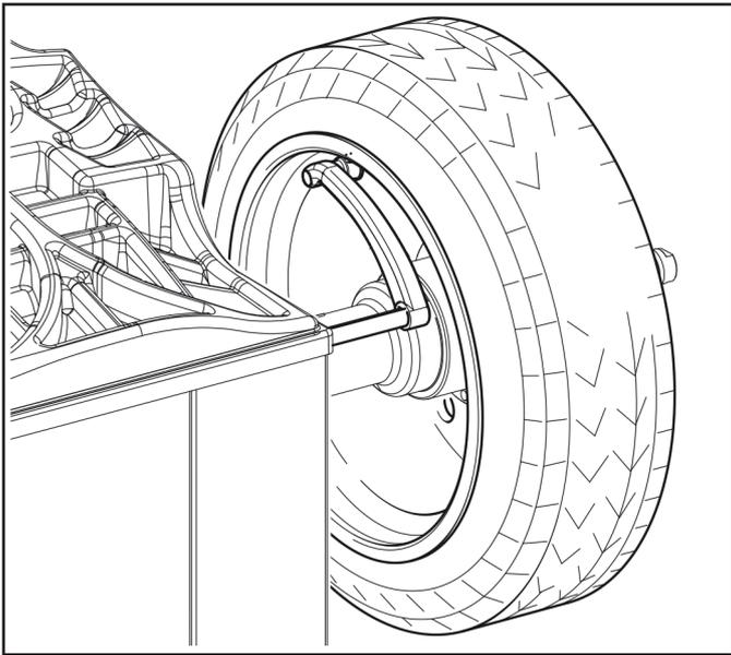
Detect the measure in mm and enter it through keys
