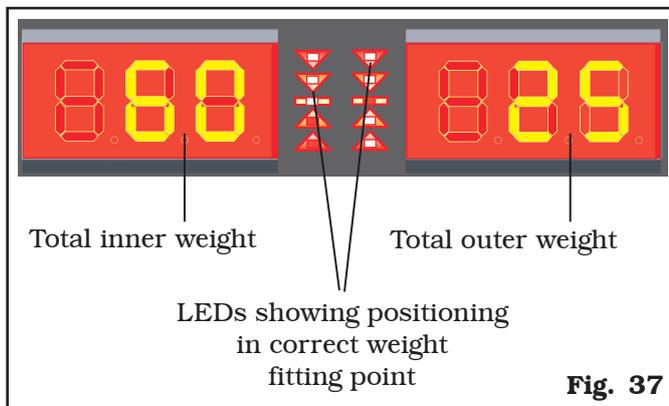
To position wheel on the OUTER side, turn it in the direction shown by the LEDs, until reaching the correct position (see Par. 15.3.6). Upon reaching the correct position, the wheel is locked automatically.
