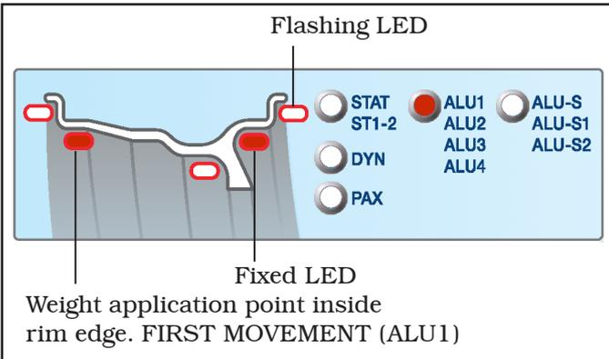
ALU2 function balances wheels with light alloy rims by fitting adhesive weights on the outside and inside of the rim. The position of the outer weight is not visible but hidden inside. Enter the measurements (see Par. 15.1) and proceed as for dynamic unbalance at 12 o’clock (both).
