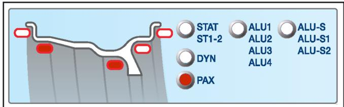
For ALU-S, STATIC, ALU1 and PAX functions, see relevant paragraphs. For all the other previously-indicated functions, wheel balancing will be done as indicated for dynamic balancing (see Par. 15.3.3). The wheel balancer will automatically correct the measurements entered by the operator according to the selected function.
