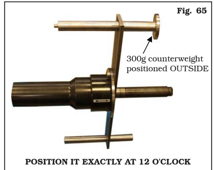
Press key to make a wheel spin with 300 g on the outer side.
