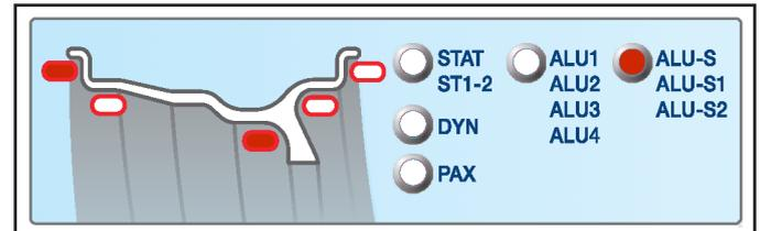
ALU-S2 function allows the balancing of wheels with light alloy rims by fitting two adhesive weights on rim outer and inner sides (both weights at "12 o'clock").
