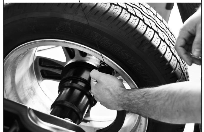
Bring the distance-diameter caliper arm into resting position.
