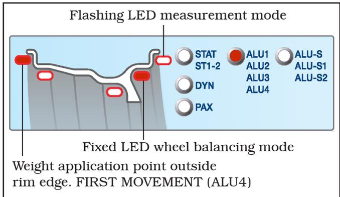
PAX function is a procedure that permits balancing PAX wheels using adhesive weights at pre-set distances to offset wheel unbalance. Select the wheel type model and proceed as described in Par. 15.4.2.
