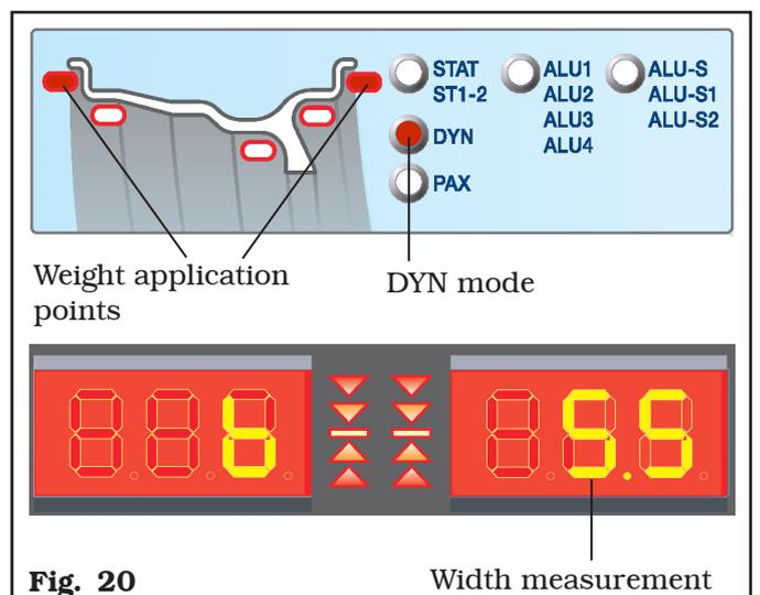
The dimensions measurement in **DYNAMIC** mode is completed.
