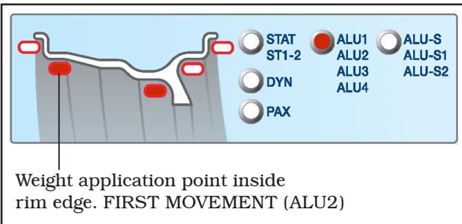
The ALU3 function is a procedure that uses mixed weights to offset wheel unbalance: weight with clip on inner side of wheel, adhesive weight at 12 o’clock on outer side, not visible because inside the rim. Enter the measurements (see Par. 15.1) and proceed as for dynamic unbalance.
