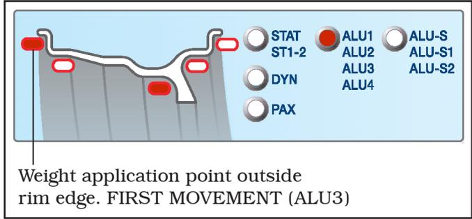
The ALU4 function is a procedure that uses mixed weights to offset wheel unbalance: weight with clip on inner side of wheel, adhesive weight on outer side “at 12 o’ clock”. Enter the measurements (see Par. 15.1) and proceed as for dynamic unbalance.
