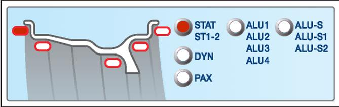
ALU1 function permits balancing wheels with light alloy rims by fitting adhesive weights on the outer and inner sides of the rim at 12 o’clock (both). Enter the measurements (see Par. 15.1) and proceed as described in Par. 15.4.1.
