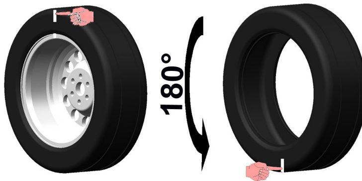
Fig. 64 Position the reference mark on the rim in line with the arrow on the flange
